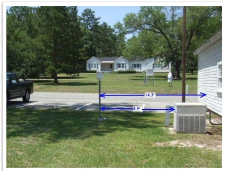
Left: USHCN climate station in Bainbridge, GA, showing the MMTS pole sensor in the foreground near the parking space, building, and air conditioner heat exchanger, with the older Stevenson Screen in the background located in the grassy area.
